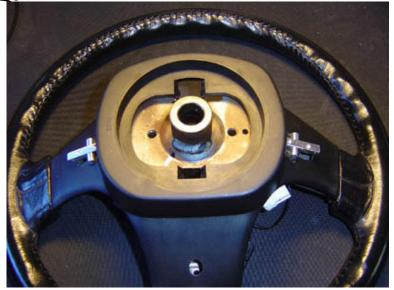
Install also the return spring before the back cover is fit in place. The spring has to rest on the spring retainer supplied, as not to slip away. The upper end of the spring is retained by the paddle mounting screw (see picture below).
